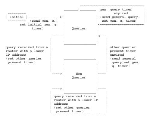
A router should start in the Initial state on all attached networks, and immediately move to Querier state.
